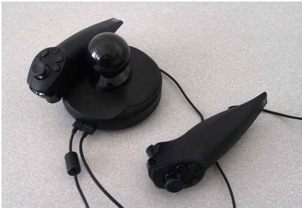
Fig. 1. The Razer Hydra game controller – central antenna and two game pads
