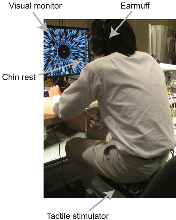
Fig. 1. Configuration of the experimental apparatus. The subject was instructed to sit on the tactile stimulator and gaze at the fixation cross at the center of the monitor. The distance between the monitor screen and the subject's face was 30 cm. Experiments were performed in a darkened room.
