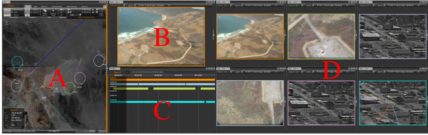
Fig. 3. Sample interface with map (A), master sensor screen (B), timeline (C), and six dedicated sensor screens (D)
