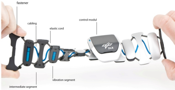
Fig. 1. The vibrotactile feedback device “VibroTac”
