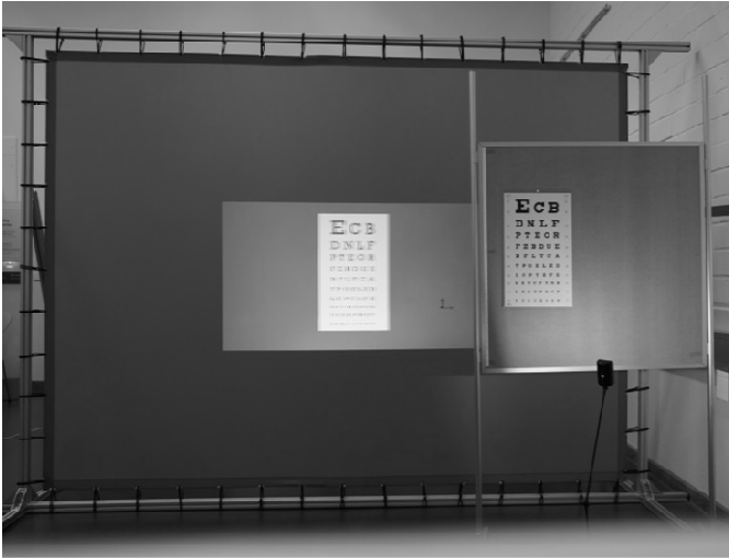
Fig. 1. Shows the physical standardized eye examination plate on the right hand side and the projected plate on the left hand side
