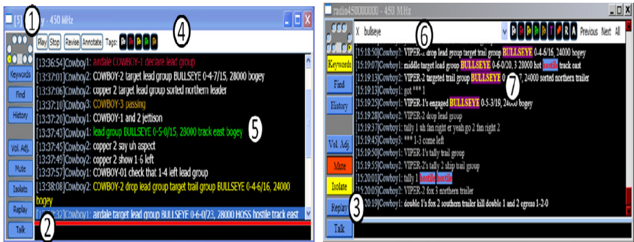
Fig. 1. Two MMC displays. 1) Spatial location of audio channel; 2) Chat input field; 3) Control buttons; 4) Playback, edit/annotate controls, and flag icon tags; 5) Flagged/Transcribed text; 6) Find control; 7) Keyword highlight.
