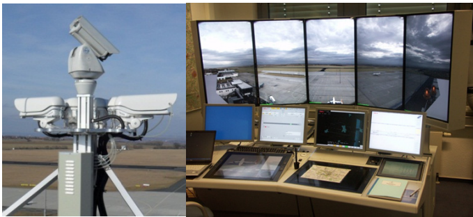
Fig. 1. Remote tower installation with 200°-panorama and pan-tilt zoom camera sensor system at the tower roof (left photo), and operators workplace with 40"-HD-format displays (right)
