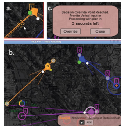
Fig. 6. Notification and Decision point behaviors showing (a) insertion of a notification point, (b) activation of that notification point and the resulting message, and (c) a similar message for a decision point
