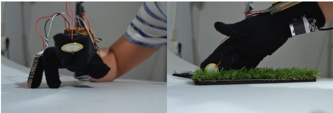
Fig. 5. Glove tangible sound generator. From textures sound is generated upon touch and stroking motions. Can even be played rhythmically.
