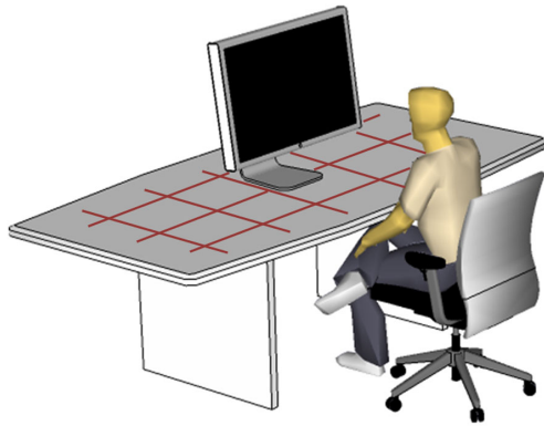
Fig. 1. The smart desk is equipped with a 3 by 5 grid of capacitive proximity sensors. The sensors measure the proximity to a user’s body parts, for example the knees placed below the table, or the hands placed upon the table.
