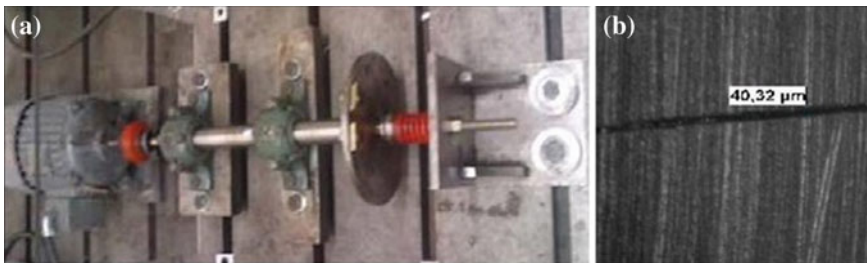
Fig. 2 a Experimental test bed. b The artificial defect of outer ring
