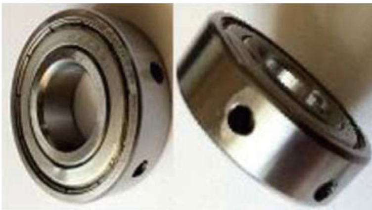
Fig. 8 Bearing with artificial fault
