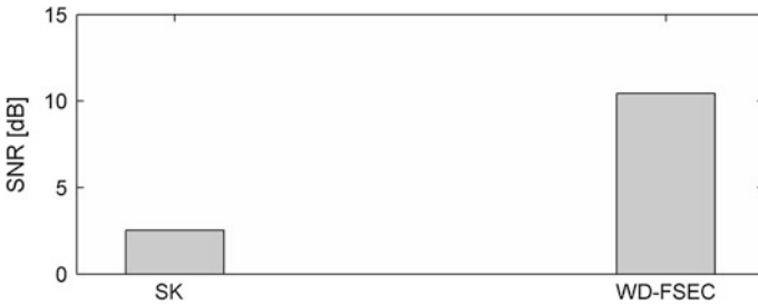
Fig. 10 SNR comparison of SK-based Envelope spectrum of the vibration acceleration signal versus FSEC
