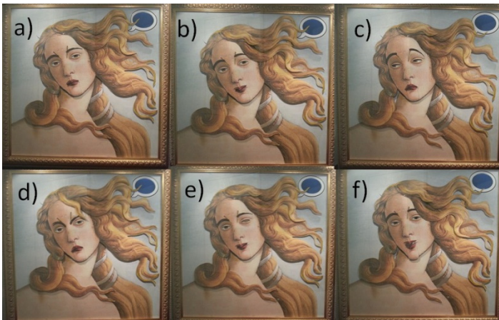
Fig. 4. Aphrodite can mime several facial expressions that are mapped on the Plutchik's wheel of emotions: a) is the neutral expression with no associated emotion; b) represents the smile for happiness; c) is frown for sadness; d) is frown and glum for anger; e) is wink for trust; f) is laugh for ecstasy.
