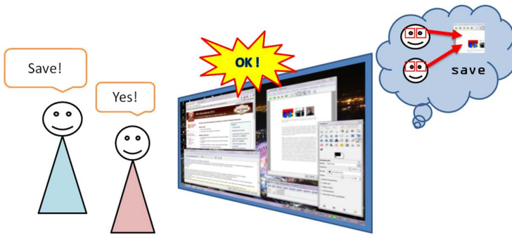
Fig. 4. When multiple browsers are opened simultaneously, it is not trivial for hands-free voice systems to understand what applications users are focusing on. The proposed system uses gaze and speech processing to determine what actions to perform.
