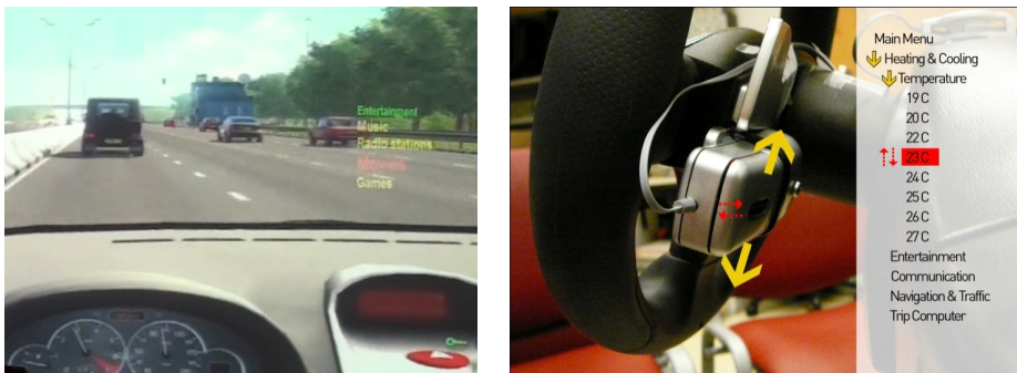
Fig. 1. The visual interface implemented as a HUD (left) and the interaction device (right). By clicking the lower mouse button (yellow highlight), the participants selected an item or descended in the hierarchy; the scrolling wheel (red highlight) was used to select an item; the upper mouse button (yellow highlight) was used for ascending in the hierarchy.
