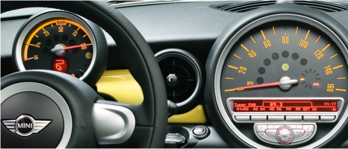
Fig. 1. MINI E dashboard (Fotocredit: BMW Group): Battery level indicator (left) and central gauge (right)
