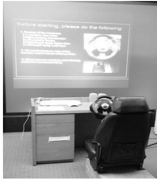
Fig. 1. STISIM Drive - Driving simulator
