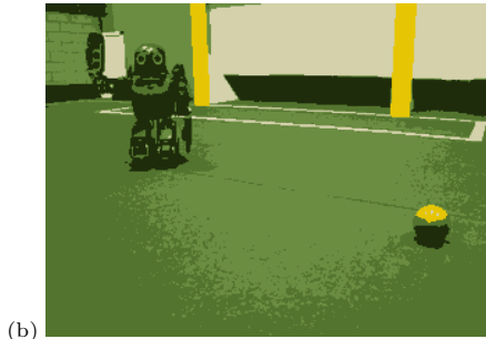
Fig. 1. Original image mapped to the corresponding five clusters for each colour space. (a) Original image; (b) 5-colour mapping using the RGB colour space; (c) 5-colour mapping using YC_bC_r ; (d) 5-colour mapping using HSV; (e) 5-colour mapping using CIELAB. For (b-e), the five colours represent the centroid of their respective clusters. Note the best performance for the YC_bC_r space, which successfully captures red, white, yellow and light green, with the black colour represented as a darker shade of green. Note also the presence of some artifacts, such as the ball being mapped into three colours: yellow, light green and dark green for RGB; and two shades of red for CIELAB.
