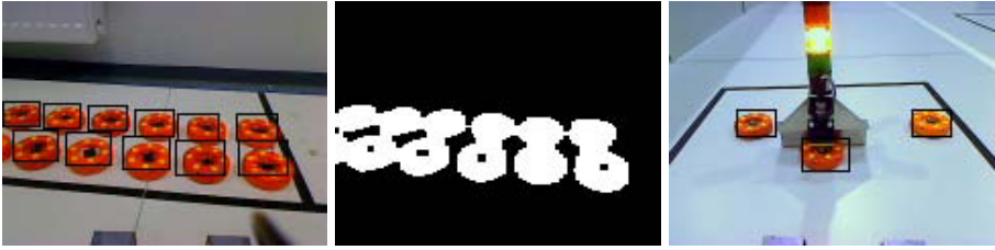
Fig. 5. Puck detection at the raw material zone (left) with the corresponding binary image (middle) and near the production machines (right)
