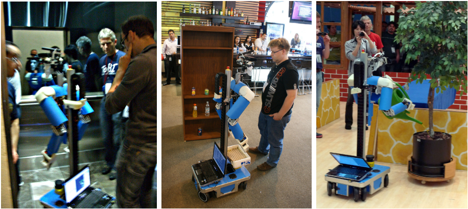
Fig. 6. Left: Cosero follows a guide into an elevator during the Follow Me test. Middle: In the Restaurant test, a guide shows Cosero drink and food locations in a real and previously unknown restaurant. Right: Cosero waters a plant in the final.
