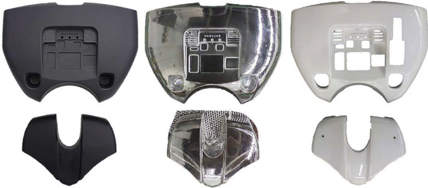
Fig. 3. (Left to right) Cover molds, vacuum formed covers, and post processed covers
