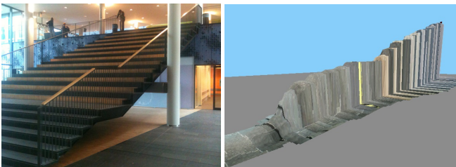
Fig. 8. Photo and map of a large stair at our university which is traversed by the AR.Drone. The depth of each step is 30 cm and the height of each step is 18 cm. The total height of the stair is 480 cm.
