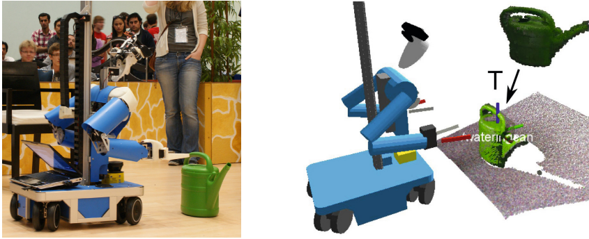
Fig. 4. Object pose tracking. We train multi-view 3D models of objects using multi-resolution surfel maps. We estimate the pose of objects in RGB-D images through real-time registration towards the model. We apply object tracking, for instance, to track the model (upper right) of a watering can for approaching and grasping it.
