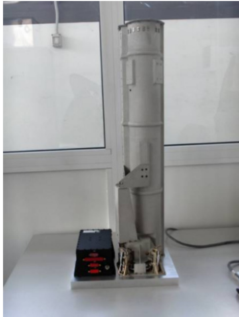
Fig. 12.26 Rosetta Drill, Sample & Distribution, called SD2 (SD2, 2012). Courtesy ESA
