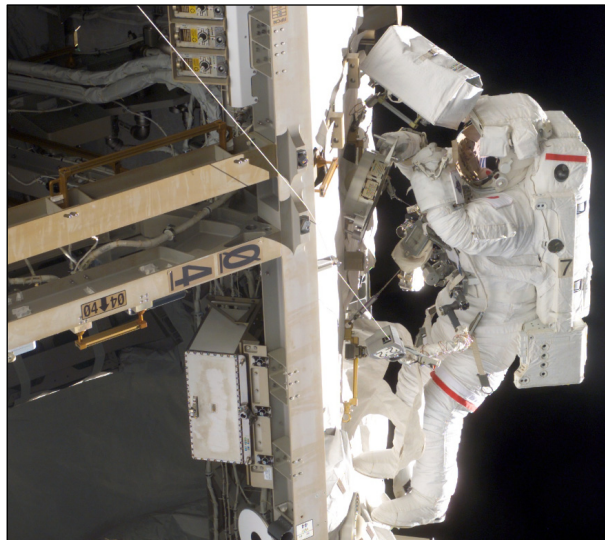
Fig. 12.11 Astronaut Soichi Noguchi, STS-114 applies a sealant to a number of test coupons during an Extra Vehicular Activity. Photo courtesy NASA.
