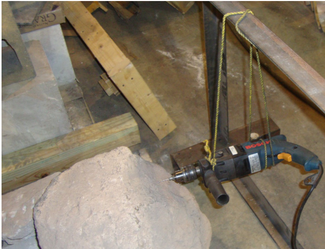
Fig. 12.9 Low WOB drilling tests in basalt
