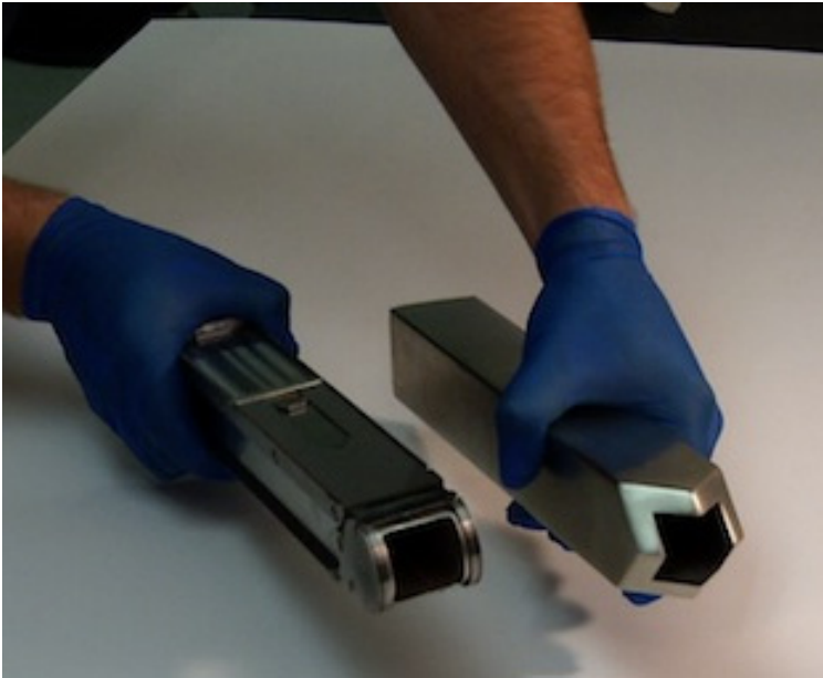
Fig. 12.35 NASA GSFC Sample Retrieving Projectile (SaRP). The photo shows a prototype sampler tip (right) and the sample collection cartridge (left).
