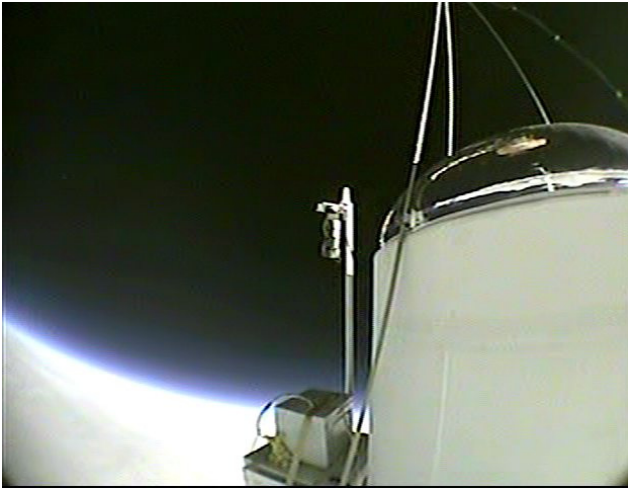
Fig. 15.10 Telemetry image of the cassette with uncured epoxy composition in stratosphere (40 km altitude)
