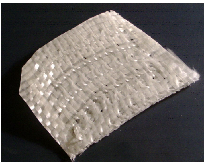
Fig. 15.3 Glass fiber composite with epoxy matrix cured in vacuum
