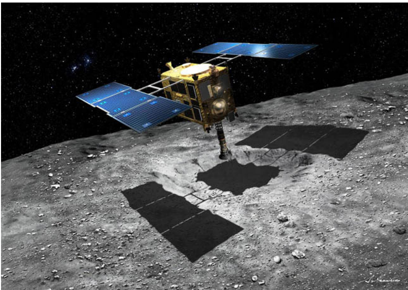
Fig. 12.5 Concept of Japan's Hayabusa 2 spacecraft. Hayabusa 2 would hurl an impactor into the asteroid 1999 JU3, sample the exposed crater material and bring it back to earth. Credit: JAXA/A. Ikeshita. http://www.space.com/14759-asteroid-sample-mission-hayabusa-2.html
