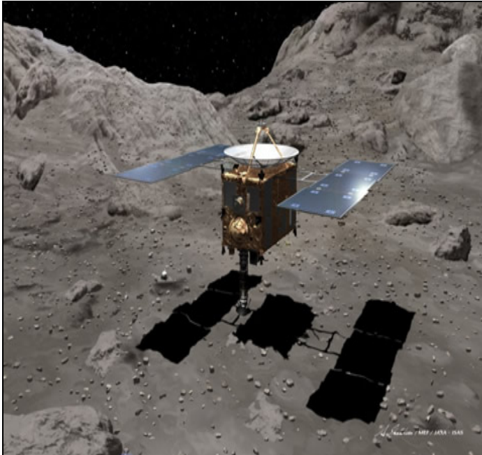
Fig. 12.24 A graphic of Hayabusa spacecraft acquiring a sample from the Itokawa S-type asteroid. Courtesy JAXA
