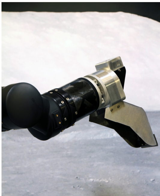
Fig. 12.43 Vibratory scoop can substantially reduce excavation forces
