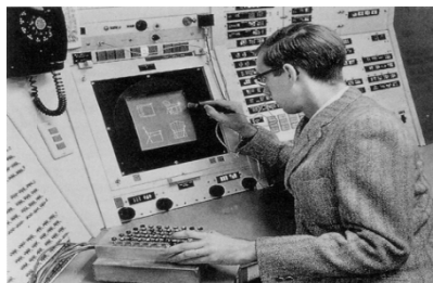
Fig. 3. Ivan Sutherland's ground-breaking Sketchpad console, 1962. Sketchpad is operated with a light pen and a command button box (under left hand) [8] - evidence of gestural interaction.
