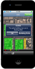
Fig. 1. This screen illustrates a rewording of a screen to enhance usability of a pop-up notification. The screen also introduces a legend or key above the tab bar for glanceable reference.
