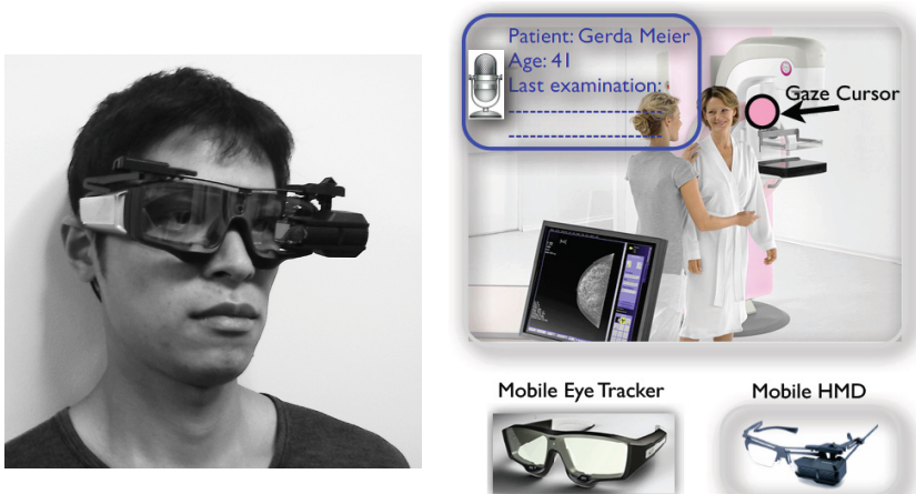
Fig. 2. Mounted eye tracker and HMD combination (left); doctor's view with HMD (right image: courtesy of Siemens AG)
