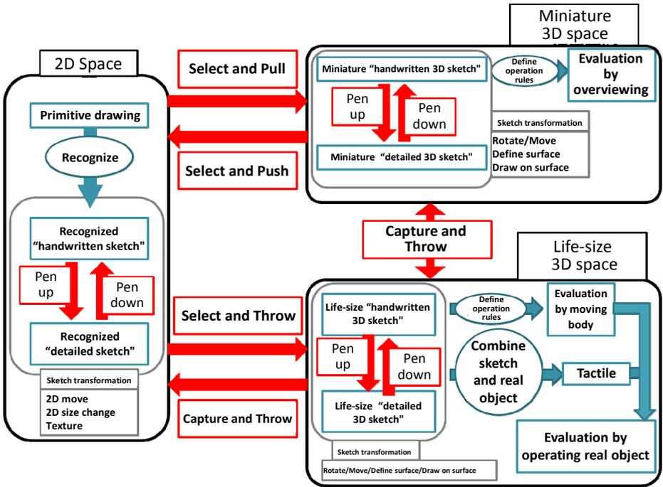
Fig. 9. New design process
