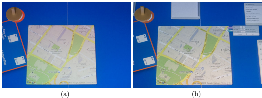
Fig. 3. (a) A cutout of an EMIL prototype in the live mode in which two documents connected to tangible objects and a map widget are visible. (b) The same cutout as in (a) but in the authoring mode. On the right of the widgets, plugs allow accessing the widgets' properties menu. For instance, the map widget shows the menu of its built-in map functionality. In the authoring mode, additional menus appear on the surface that allow to add widgets, behaviors and views to the prototype.
