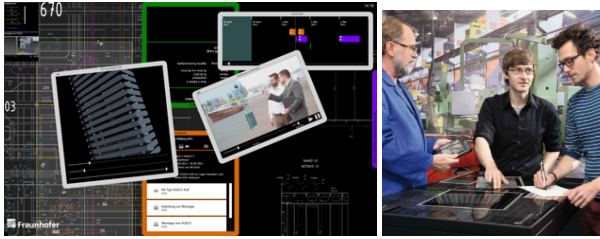
Fig. 1. Plant@Hand multi-touch user interface with linked information and in use during a team discussion
