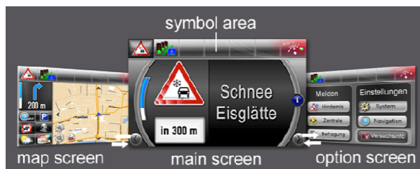
Fig. 3. Illustration of the \text{sim}^{\text{TD}} HMI depicting three virtual screens and symbol area
