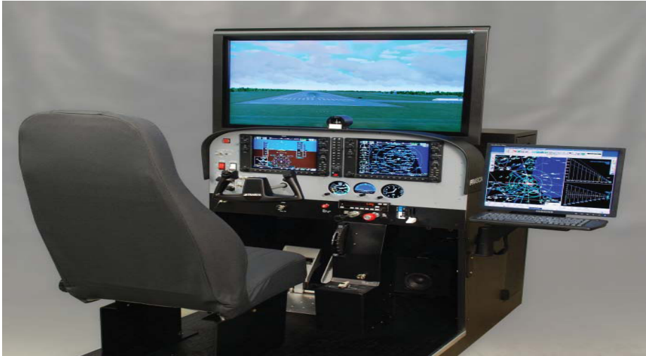
Fig. 1. Frasca Mentor Advance Aviation Training Device (AATD). The training device replicates the cockpit of the Cessna 172, G1000 configuration (Frasca, 2010).
