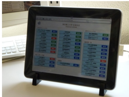
Fig. 7. Display and auto refresh of presence on tablet device
