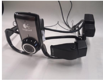
Fig. 4. Device NWEBcamera: Logicool 2-MP Portable Webcam C905m, HMD: SCALAR Teleglass-3 T3FCEMA
