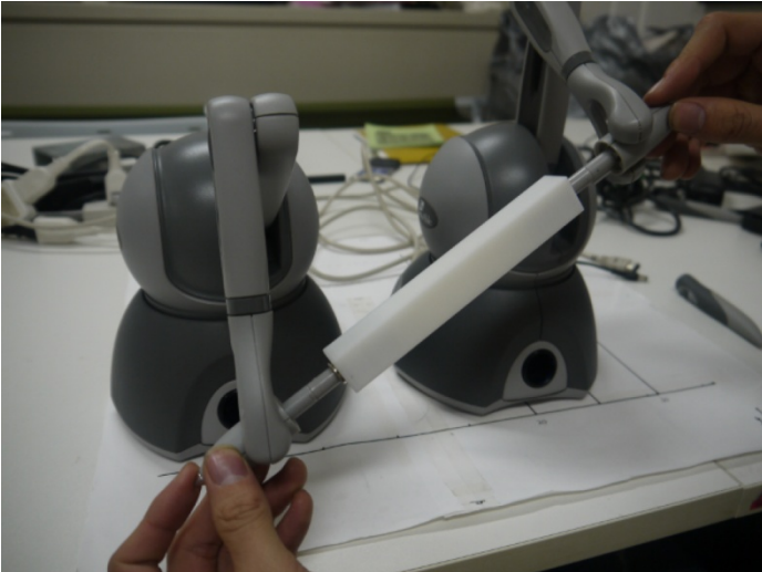
Fig. 2. Two haptic devices connected by connecting bar
