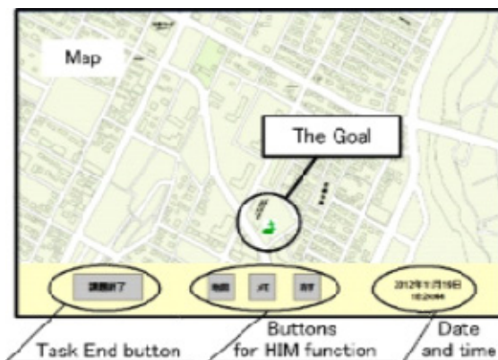
Fig. 1. Screen of specific digital map with touch panel
