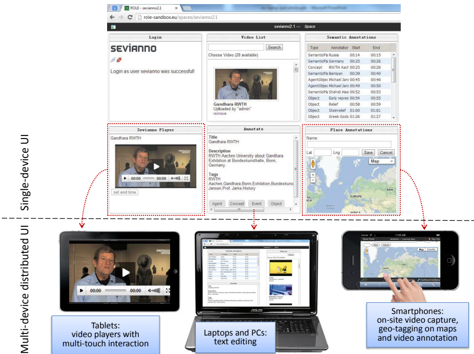
Fig. 1. An example of distribution of user interface components (widgets) to diverse (mobile) computing devices
