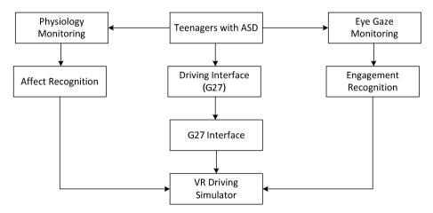
Fig. 1. System diagram of the adaptive driving platform
