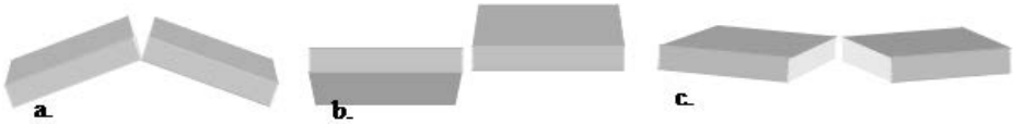
Fig. 1. Keyboard adaptations to reduce postures: a) roll angle (pronation/supination); b) pitch angle (wrist flexion/extension); c) yaw angle (wrist ulnar/radial deviation)
