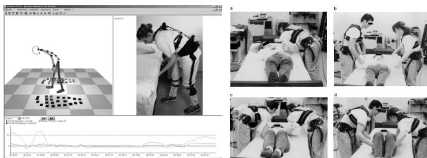
Fig. 2. CUELA measurement system, LMM and EMG systems in use [6], [13]
