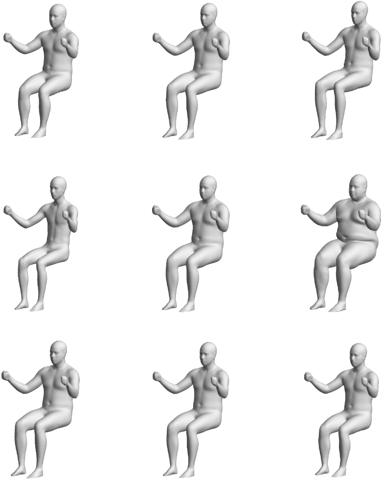
Fig. 5. Anthropometric effects. Top row: Stature 1600 to 2000 mm. Middle row: BMI 18 to 40. Bottom row: ratio of sitting height to stature 0.48 to 0.56.
