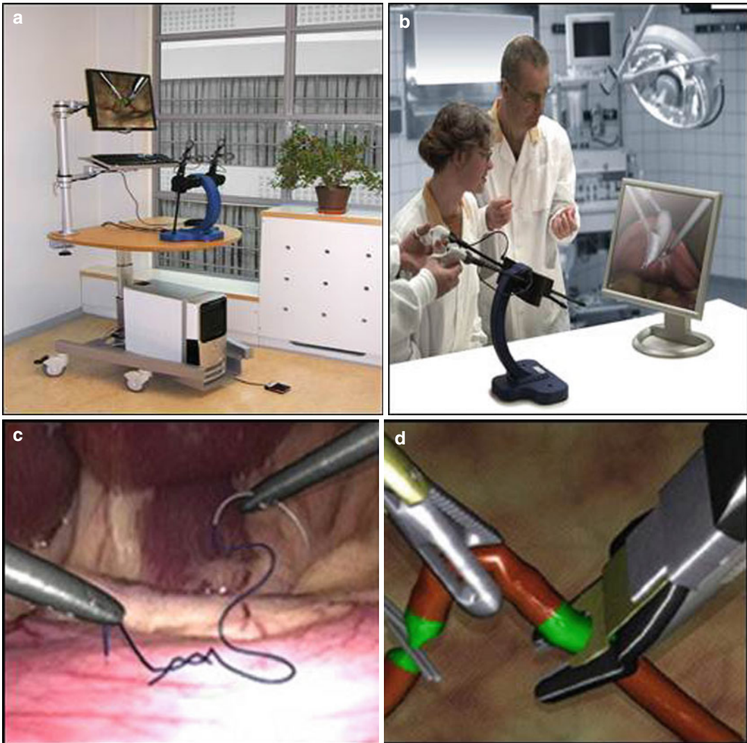
Fig. 8.14 (a) LapSim® – device with the Immersion Medical interface, a graphic design of the sewing (b) and clip application task (c) (Courtesy of Dr. Iyad Haasan)
