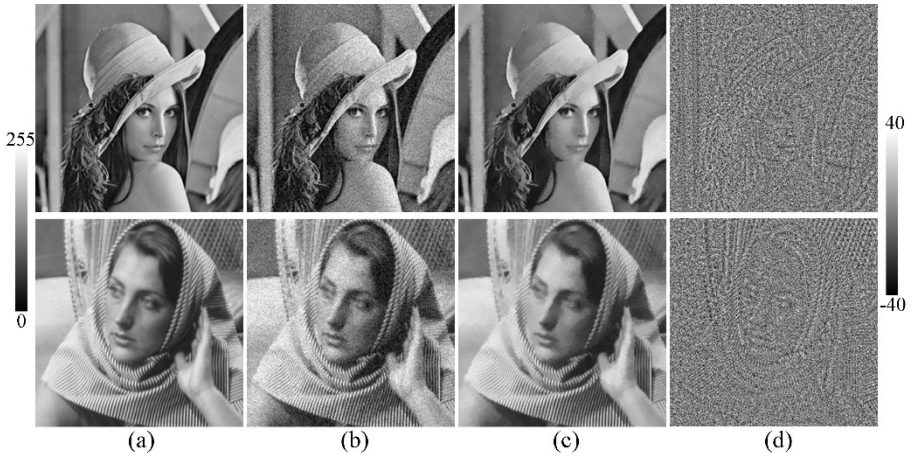
Fig. 1. Denoising results of NLM and corresponding residual image. (a)ground truth; (b)noisy image (original image) with noise level 7%; (c) denoise image; (d)Residual image.
