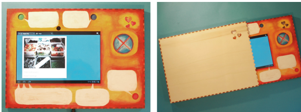
Fig. 3. Integrated TabletCompanion with 10-inch display (left and right). The device features several quick access buttons and space for notes by the users. It comes with a wooden casing (right) for easy and appealing storage.
