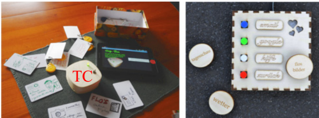
Fig. 2. Black, 7-inch tablet computer with Wireless TabletCompanion and various RFID tokens (left). Wired TabletCompanion with four quick access buttons and three RFID tokens (right).
