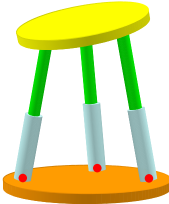
A 3D Platform: All joints connected to both the top and base discs are ball-joint, and each prismatic joint can also be spinning.
