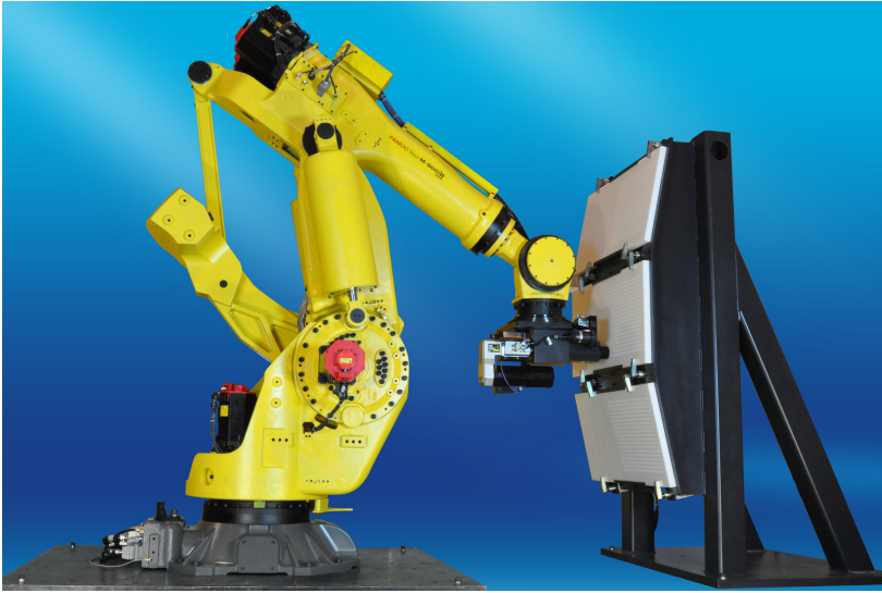
Fig. 1.2 A Fanuc M-900iB/700 industrial robot in drilling operation. Photo courtesy of Fanuc Robotics, Inc.
