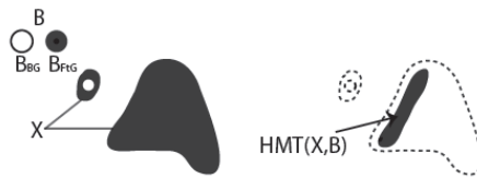
Fig. 3. An example of a hit-or-miss transformation. It shows that it is necessary for both reference points to meet at the desired target for the operation to be performed, otherwise a gap appears in the region of the resulting image (Taken from [19]).
