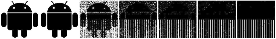
Fig. 4. A Droid-bitmap in RAM of a Galaxy Nexus device after 0, \epsilon , 0.5s, 1s, 2s, 4s, and 6s without power. The cold boot attacks have been deployed at room temperature.
