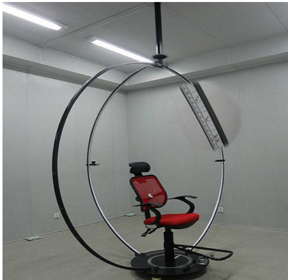
Fig. 29.5 Sound source positioning system of HRTFs measurement
