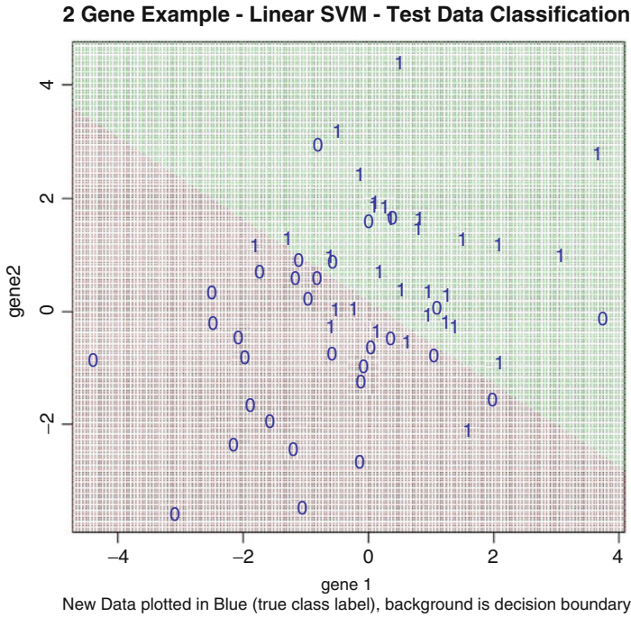
Fig. 6.13 The decision regions of the linear SVM based on the simulated training data set, along with the actual class labels of the simulated test data set
