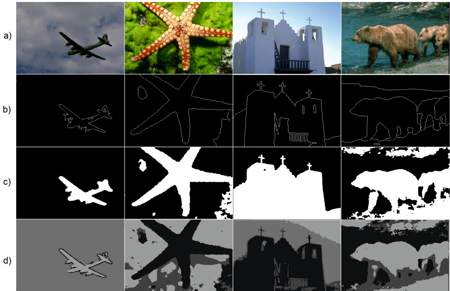
Fig. 1. Segmentation results: a) Original image, b) Ground truth, c) Results the of proposed method with K = 2 , d) Results of the proposed method with K = 4
