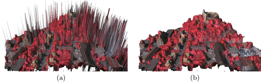
Fig. 1. Range image integration results on the ISPRS Vaihingen test dataset [2]. (a) Fused DSM computed by median fusion, which shows considerably non-robust results. Single isolated outliers are still present in the results. (b) Our probabilistic fusion approach effectively discards outliers and produces visually clean results.
