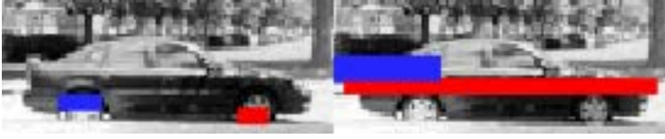
Fig. 5. 2Rec-Features selected by the AdaBoost algorithm in the application of lateral car detection
