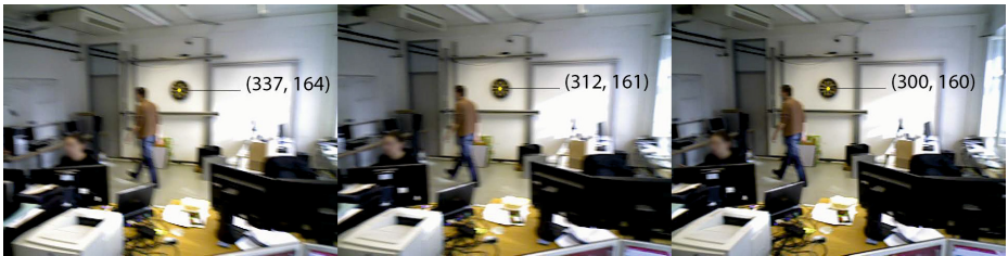
Fig. 1. Three consecutive frames using a moving camera. The coordinates of the centroid of the dartboard are taken to demonstrate the amount of movement between frames.
