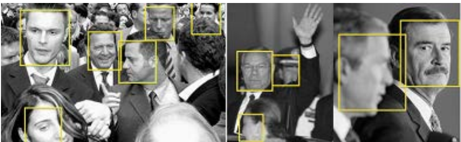
Fig. 6. Example detections on the FDDB [24]. Lateral or partially occluded faces are detected.
