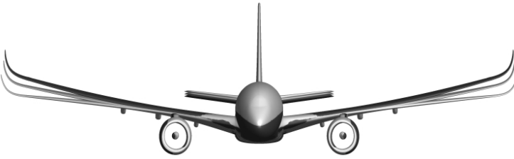
Fig. 10. Comparison of jig, 1g-, and 2.5g flight shape for a generic full aircraft configuration
