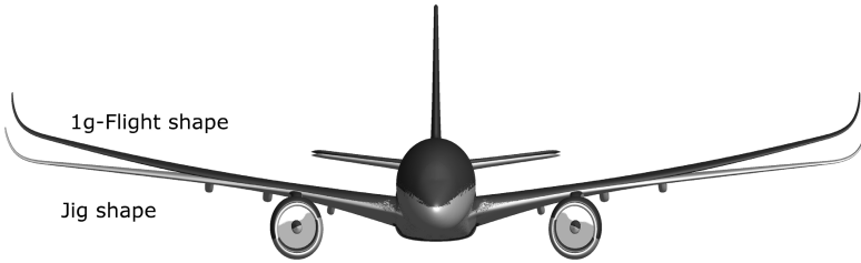
Fig. 4. Front view of the jig and calculated 1g-flight shape for a generic full aircraft configuration
