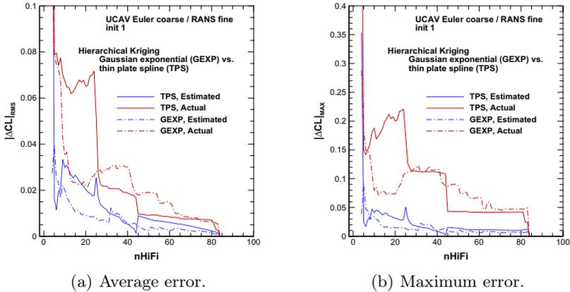
**Fig. 13.** Convergence of  $C_L(M, \alpha)$  surrogate model for UAV test case; average error on data points. High-fidelity model: fine grid Navier-Stokes; low-fidelity model: Euler simulation (coarse grid). Comparison between Gaussian exponential and 'thin plate spline' Kriging correlation functions.
