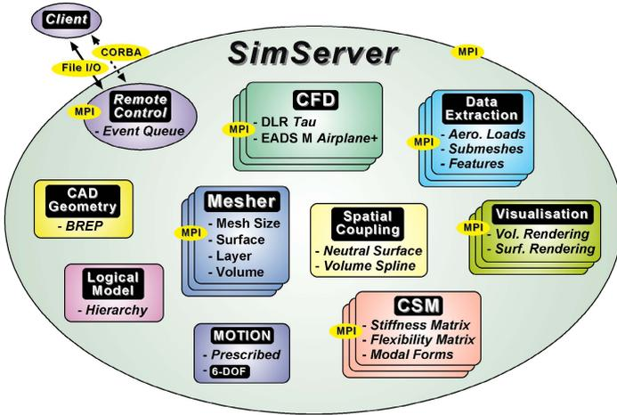
Fig. 1. Modular architecture of Cassidian *SimServer* simulation environment [8]
