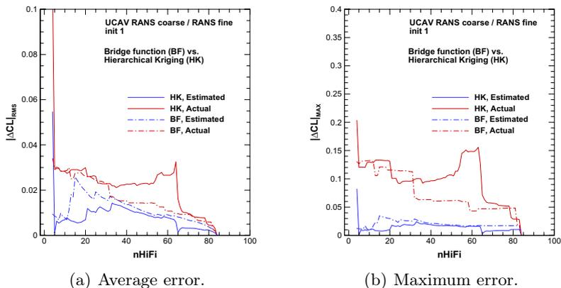
**Fig. 15.** Convergence of  $C_L(M, \alpha)$  surrogate model for UAV test case; average error on data points. High-fidelity model: fine grid Navier-Stokes; low-fidelity model: coarse grid Navier-Stokes. Comparison between Kriging with bridge function (BF) and hierarchical Kriging (HK) multi-fidelity approaches.
