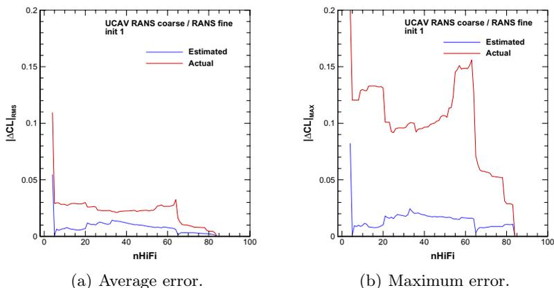
**Fig. 9.** Convergence of  $C_L(M, \alpha)$  surrogate model for UAV test case. High-fidelity model: fine grid Navier-Stokes; low-fidelity model: coarse grid Navier-Stokes.
