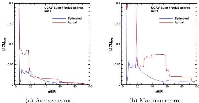
**Fig. 8.**  $C_L(M, \alpha)$  surrogate model for UAV test case, based on Navier-Stokes simulation (coarse grid) as high-fidelity model and Euler simulation as low-fidelity model. Convergence of the model error with the number of high-fidelity points. Red: actual error of surrogate model to high-fidelity data; blue: estimated error (MSE) of the hierarchical Kriging interpolation.
