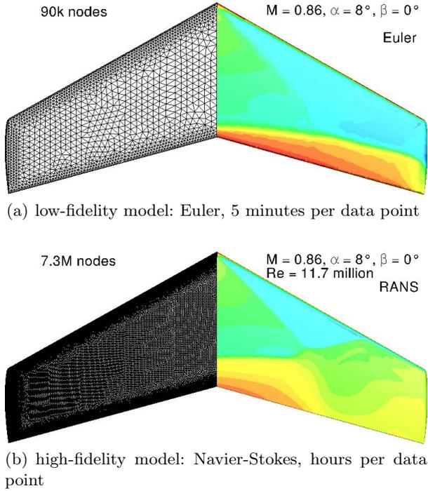
**Fig. 3.** Euler and Navier-Stokes simulation for the ONERA M6 wing at  $M = 0.86$ ,  $\alpha = 8^\circ$ , Reynolds number 11.7 million. Surface mesh and pressure distribution.
