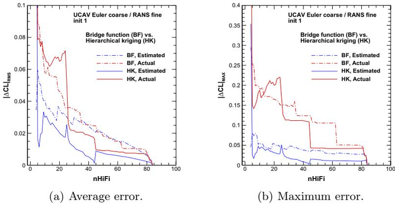
**Fig. 14.** Convergence of  $C_L(M, \alpha)$  surrogate model for UAV test case; average error on data points. High-fidelity model: fine grid Navier-Stokes; low-fidelity model: Euler simulation (coarse grid). Comparison between Kriging with bridge function (BF) and hierarchical Kriging (HK) multi-fidelity approaches.
