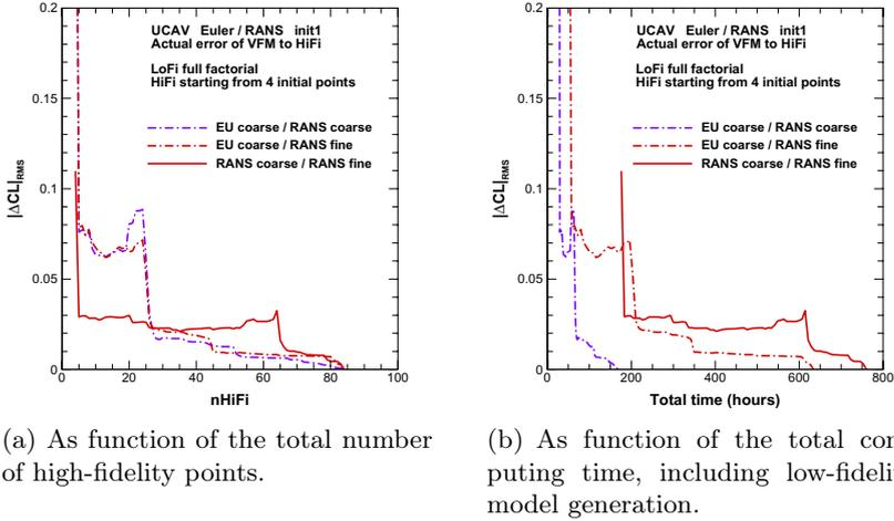
**Fig. 12.** Convergence of  $C_L(M, \alpha)$  surrogate model for UAV test case; average error on data points. Comparison between coarse grid Navier-Stokes and Euler simulation as low-fidelity model.
