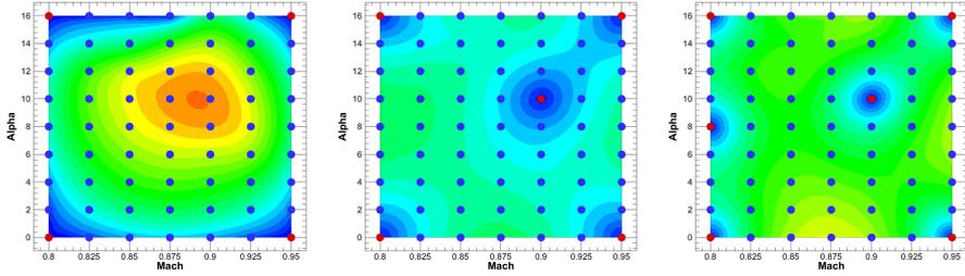
**Fig. 2.** Adaptive sampling in the  $(M, \alpha)$  parameter space. The low-fidelity data (blue dots) have been previously computed in all defined grid points (full factorial). High-fidelity data (red dots) are iteratively selected in that grid point where the estimated model error (MSE) of the multi-fidelity surrogate model, shown by the colour contours, is the highest.
