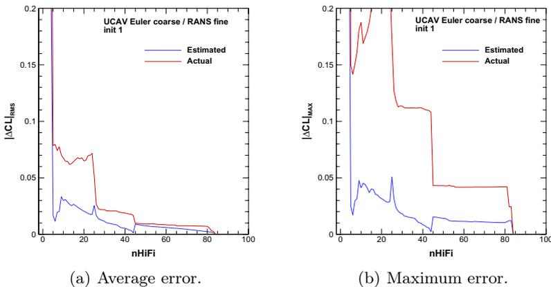
**Fig. 10.** Convergence of  $C_L(M, \alpha)$  surrogate model for UAV test case. High-fidelity model: fine grid Navier-Stokes; low-fidelity model: Euler simulation (coarse grid).
