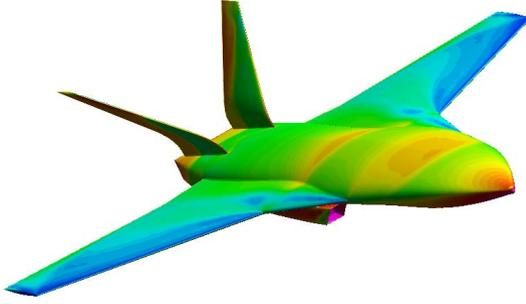
**Fig. 5.** Generic UAV configuration as test case for the adaptive sampling method with *Simserver* and the *SMART Toolbox*. Pressure distribution at Mach number 0.95 and  $15^\circ$  angle of attack; Navier-Stokes simulation on coarse grid.
