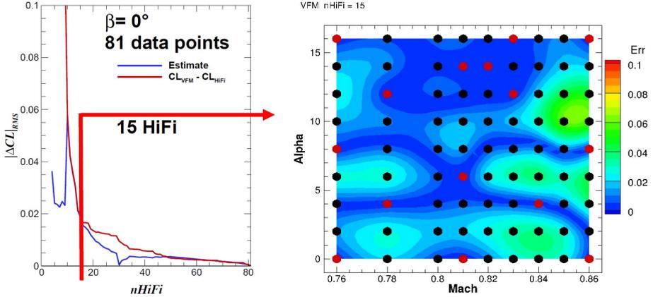
**Fig. 4.** Construction of  $(M, \alpha)$  data set for the ONERA M6 wing using Euler / Navier-Stokes multi-fidelity simulation. Left: convergence of the actual error of the surrogate model with the number of high-fidelity points. Right: sampling in the  $(M, \alpha)$  parameter space with 15 high-fidelity points and the corresponding MSE error estimate.
