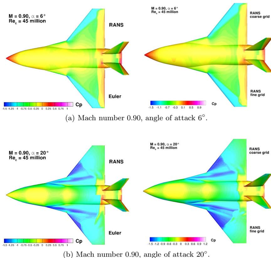
**Fig. 6.** Comparison of pressure distributions computed with models of different fidelity. Left: coarse grid Navier-Stokes versus Euler; right: coarse versus fine grid Navier-Stokes.
