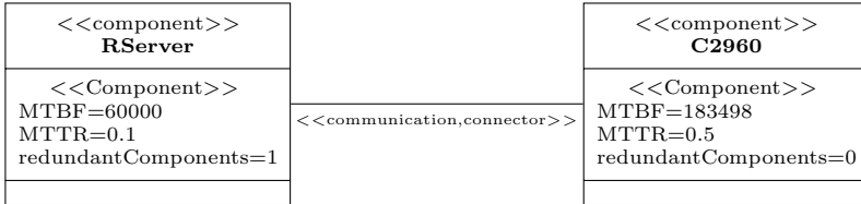
Fig. 7. Predefined network elements represented in UML Class Diagram
