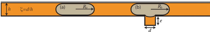
Fig. 2.6 Sketch of the droplet above the anchor and far away. The channel height is h , the hole diameter is d and its depth is e
