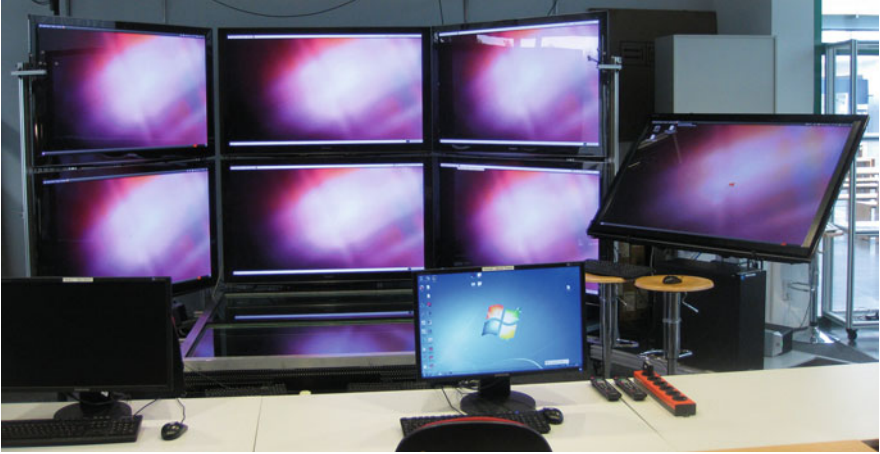
Fig. 3 General FRAVE setup: three walls in bended power-wall setup with adjacent tiltable display and remote desktop computers in front of FRAVE
