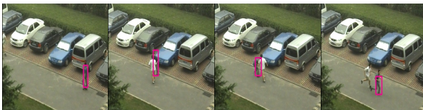
Fig. 6. Tracking result of the target having large blocking area by proposed algorithm, from left to right are respectively the frame of (a) 80 th , (b) 311 th , (c) 362 th , (d) 452 th
