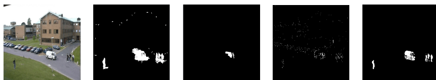
Fig. 3. Detection result of different algorithms, from left to right are respectively (a) a frame of scene 1, (b) detection result of mixture Gaussian model, (c) detection result of Bayesian decision, (d) detection result of three frame subtraction, (e) detection result of codebook.
