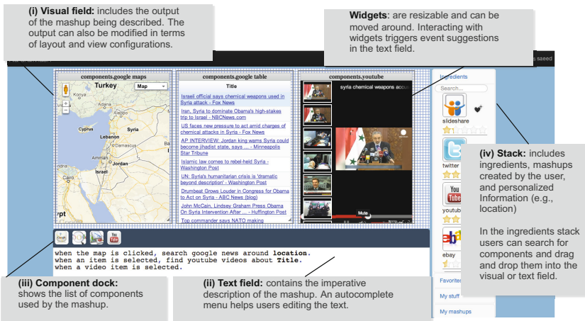
Fig. 1. NaturalMash environment: the ingredients stack gives an overview of the tool functionalities (available mashup components). From there, users can drag-and-drop ingredients to start building mashups. Alternatively, they can use the text field to discover desired components. With the help of the autocomplete menu, users type in the text field the imperative description of the mashup in natural language, and immediately see the result in the visual field.
