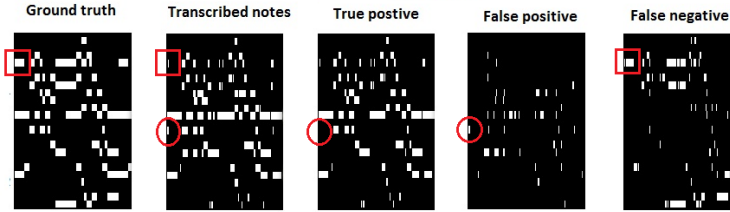
Fig. 2. This figure illustrates our pixel based evaluation scheme. This approach calculate TP, FP, and FN from the number of pixels. The three squares highlight a false negative example and the three circles highlight a false positive example.
