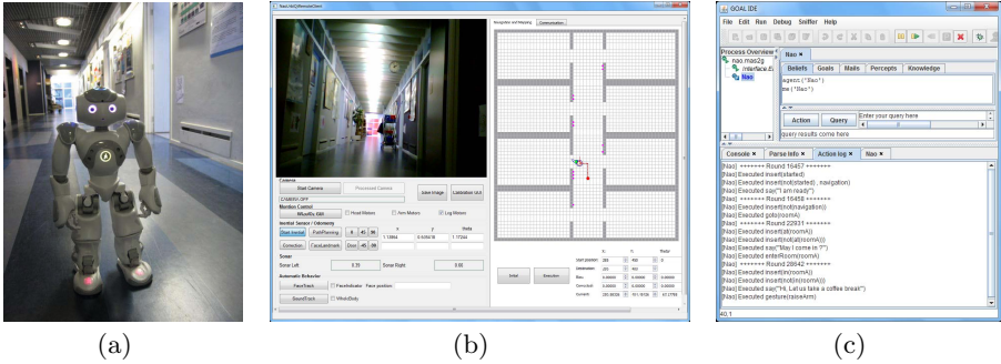
Fig. 3. The navigation task: (a) humanoid robot NAO, (b) the GUI of the robotic behavior layer, (c) the cognitive reasoning in GOAL
