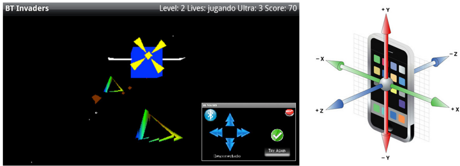
Fig. 3. Mobile-mobile game application. Left: The center image shows the 3D rendering of the display device running. The lower-right-hand corner presents the customized interface of the controller device. Right: Mobile accelerometers for [x,y,z] axes.
