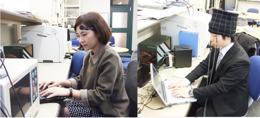
Fig. 1. Brain NIRS measurement under typing
