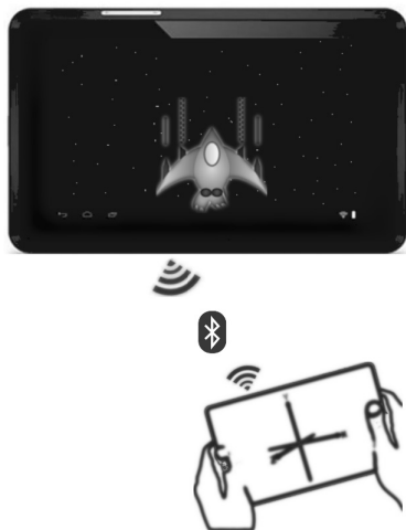
Fig. 2. Game concept of the mobile-mobile application. At the top, the display device rendering the graphic part of the game and receiving commands from the controller application through Bluetooth (at the bottom).
