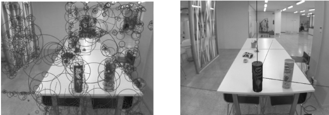
Fig. 3. Left: object detection using texture. Right: object tracking using edges.
