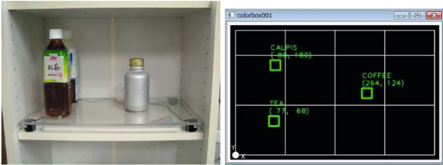
Fig. 2. Information about objects provided by the intelligent cabinet. Squares in the screen indicate the position of the different objects together with their description.
