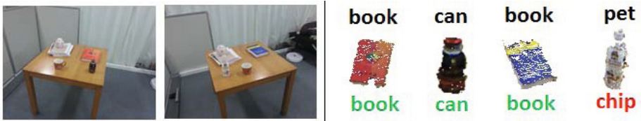
Fig. 9. Resulting matching of changes on a table. The top row indicates the label of the changed objects. The bottom row shows the categorization using our method. The pet bottle is misclassified as a chip container.
