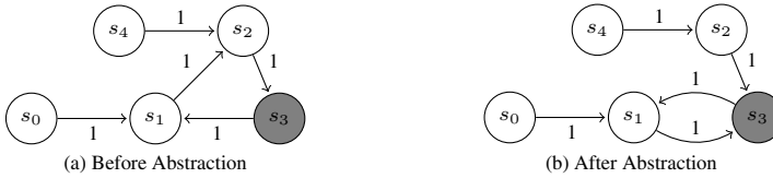
Fig. 4. Destruction of SCC during Abstraction
