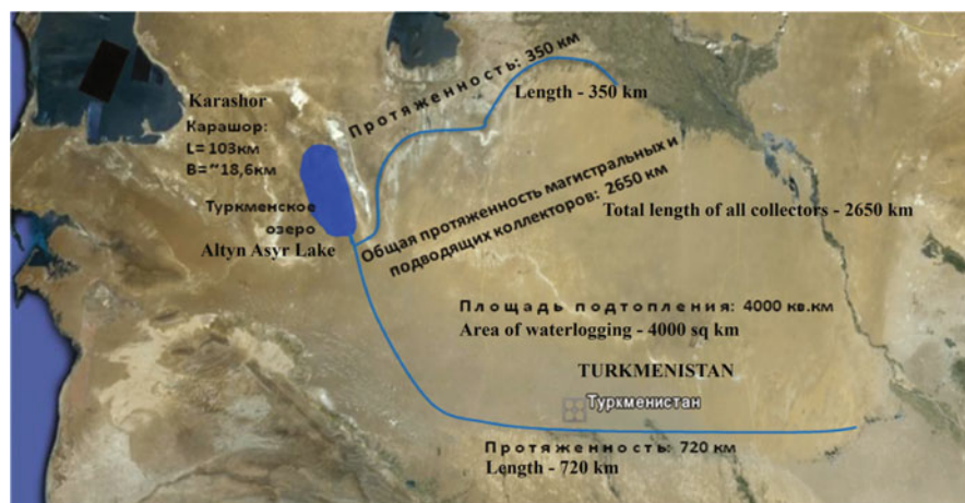
Fig. 1 Scheme of transfer of the collector and drainage waters into the Altyn Asyr Lake
