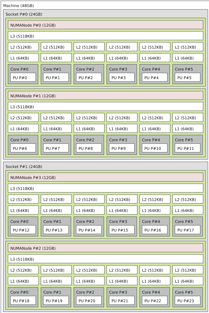
Fig. 3 Micro-architecture of computer with dual-AMD Opteron™ 6164 HE
